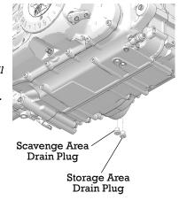
6. Reinstall the drain plugs. Torque to 15 ft. lbs. (20 Nm).
