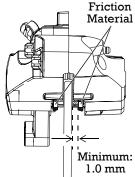
When checking brake pad friction material thickness, check each brake caliper for dampness or stains from leaking or dried brake fluid. If inspection reveals signs of fluid leakage, do not operate the vehicle. See your dealer for service.
