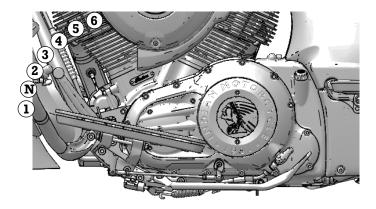
Press downward on the toe lever to shift to a lower gear. Lift upward on the toe lever to shift to a higher gear. Release the clutch lever after each gear shift. Shifting to neutral is easiest if the motorcycle is rolling slowly. To shift from first gear to neutral, gently lift the toe lever a half stroke.
