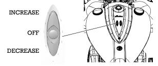
The heaters have10 heat levels, ranging from OFF (level 0) to highest heat (level 10). Press and release the top of the switch to increase the heat level by one increment. Press and release the bottom of the switch to decrease heat by one increment.
