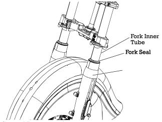
2. Clean the fork tubes to remove bugs, tar or buildup which may cause seal wear or leakage. Inspect the outer surfaces of the inner fork tubes for scratches or damage from foreign objects.
