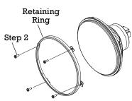
2. Remove the four screws securing the headlamp retaining ring. Remove the retaining ring.
