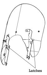
**WARNING!** Improper windshield installation can result in loss of control, accident and driving hazards for other motorists (if windshield falls from the motorcycle). Always make sure the windshield is fully seated before engaging latches.
