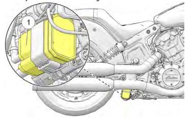
Inspect connections at the evaporative emissions canister to be sure they are secure.
