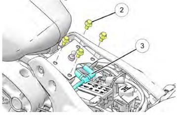
5. Disconnect the fuel tank vent line and recess drain line ③ at the rear of fuel tank.
