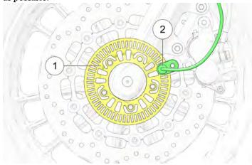
Inspect for debris adhering to the end of the wheel speed sensors ②. If contamination is observed, or if you are unable to visually inspect, slide a thin towel across the face of the sensor between the sensor and the tone ring to remove any potential debris.
