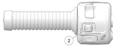
To activate the hazard switch, press on the center of the turn signal switch @.
