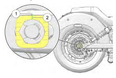
2. On right side of motorcycle, remove the c-clip ③ and loosen the axle nut ④. Retighten to **Adjustment Specification**.
