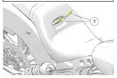
1. Remove the bolts on the back of the seat 1 using the included uni-tool.
