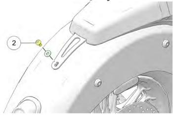
3. Grasp the front edge of the seat and pull upward abruptly to disengage the seat base grommet from the seat mount stud 3.
