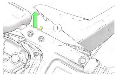
1. Grasp the front edge of the seat and pull upward abruptly to disengage the seat base grommet from the seat mount stud ①.
