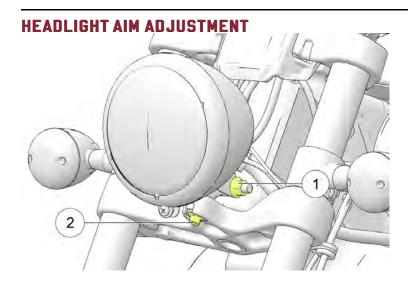
1. To adjust the headlamp vertically, loosen the housing mount fastener ① and pivot the housing upward or downward. Tighten the fastener.
