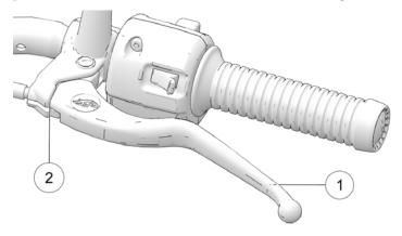
Freeplay (gap) is the amount of lever movement from the rest position to the point of cable resistance. Clutch lever freeplay should be 0.5-1.5 mm. Measure the gap between the clutch lever and the lever housing ②. See page 88. Adjust clutch lever freeplay if necessary.
