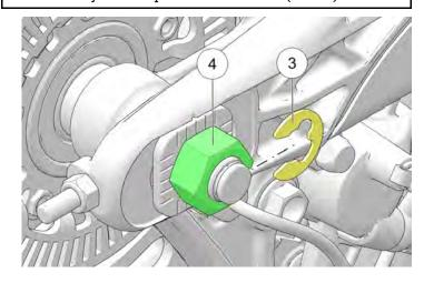
3. Turn **LEFT SIDE** adjuster nut (5) to achieve proper belt tension.
