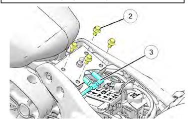
8. Connect the fuel tank vent line and the fuel cap recess drain line (3).
