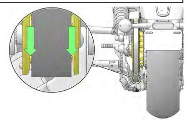
Rotate wheel FORWARD and verify sprocket teeth are still visible on both side of drive belt. If necessary, loosen axle nut and RIGHT SIDE adjuster until belt moves off left flange and begins to track down center of driven sprocket flange during forward wheel rotation.
