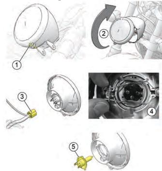
7. Reinstall the rubber boot, making sure it seals around the bulb and headlight.
