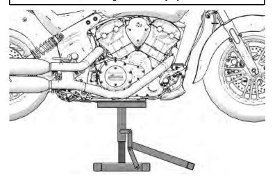
Position motorcycle platform jack beneath engine case, avoiding oil drain plug, and lift motorcycle so front wheel is off ground. Stabilize motorcycle in upright position with tie-down straps (or equivalent). Motorcycle MUST be stable prior to performing belt maintenance procedures.
