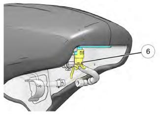
Gently feed fuel rail end of the fuel hose toward the center of the vehicle. Ensure the hose and connector are clear of coolant hose and all wire harnesses.
