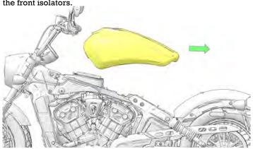
11. Lift the fuel tank off the motorcycle and place on a suitable flat surface to prevent tank damage.
