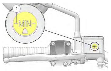
The fluid level should be above the minimum indicator mark in the sight glass.
