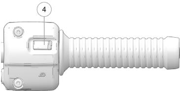
Use the Mode switch to set the display units to either standard or metric units of measurement. See the *Multi-Function Display (MFD)* section for details.
